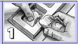
Castaldo Silicone Molding Rubber is soft and pliable, with a consistency like putty or molding clay.
