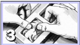
Curing Castaldo Slicone Jewelry Molding Rubber Molds involves no mixing, limited working times or de-bubblizing. Simply put it in your vulcanizer at 330°-150°F (165°-177°C) for 15 minutes per 1/4 inch (6mm).
