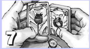
Finished molds can be simple or complex with cores, straight plugs or even spiral plugs. Castaldo Silicone Jewelry Rubber Molds are strong and tear resistant and can last for years and years.
